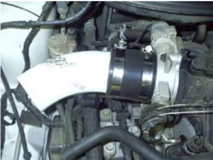
Next, put this whole assembly in place on the throttle body and lightly tighten the throttle body hose clamp.
