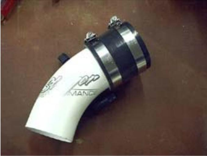
The 3" ID side of the connector fits onto the intake tube, and the 3.25" ID side connects to the throttle body. Put the connector in place on the intake tube and tighten the hose clamp.
