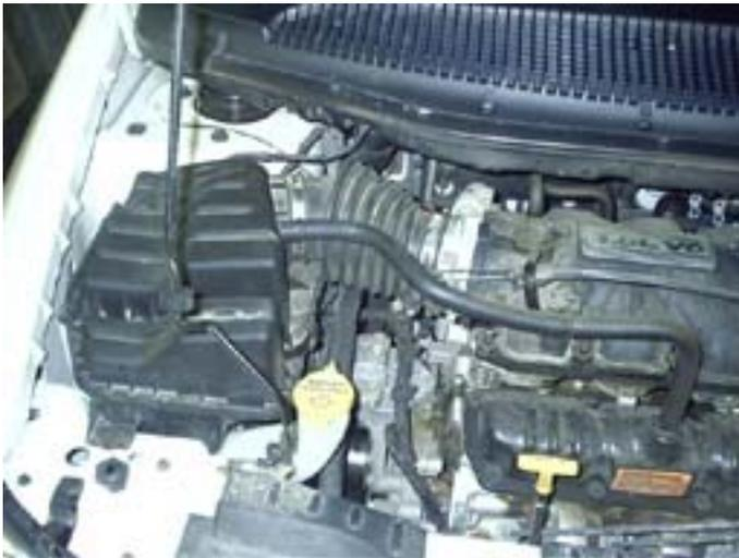
This is what we're starting with; a bone stock engine bay. The first step is to disconnect the negative battery cable. This will help to prevent any potential electrical problems, and also will "reset" the PCM so that the computer will be able to "re-learn" the engine with the new intake in place. To disconnect the battery cable, you will need a 10mm socket or wrench. (Note that this may erase your radio station presets, so you might want to write them down first, just in case.)
