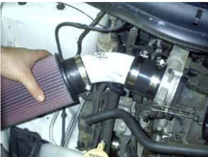
After removing it from its plastic bag, put the filter on the end of the tube and tighten that hose clamp. Now that everything is in place, you can move the intake around, loosen and rotate the hose clamps, etc. to get everything just the way you want it. You should probably check to be sure that the filter isn't resting on the fender because constant rubbing will wear away the paint. Once you get everything in its proper place and orientation, tighten down all of the hose clamps.
