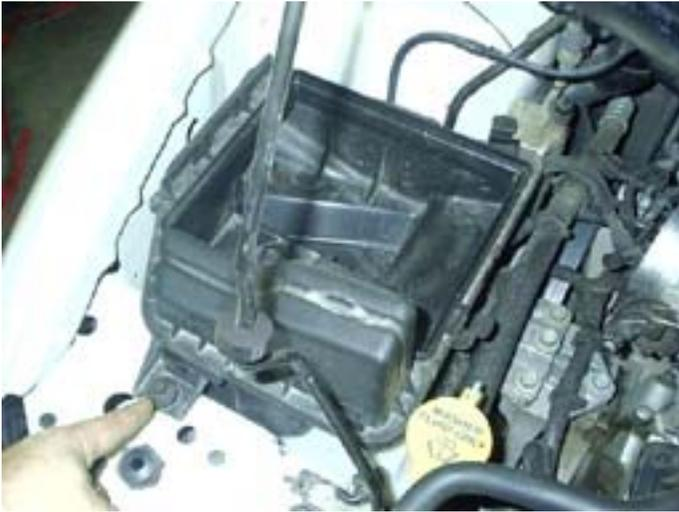
Once you have removed the 10mm hex head screw at the front of the airbox (pictured at left), you will be able to grab the airbox and pull straight up to remove it from the engine bay. (There is a post in the bottom of the airbox which looks like a bolt, but it really isn't – the airbox is designed to just pull up off of that post.) After removing the airbox, you might want to replace the screw, just to be certain that it won't get lost.
