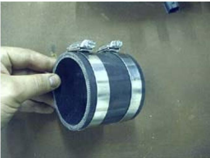
Next, assemble the silicone connector as shown at left. There are two silicone pieces, one is 3" in length with a 3.25" ID and the other is 1.5 " in length with a 3" ID. The smaller piece fits inside the larger one. What you will end up with is a connector with a 3" ID at one end and a 3.25" ID at the other. (Note: This connector is normally pre-assembled for you; I have included the above info simply for reference.)
