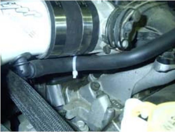
Connect the PCV hose to the nipple on the intake tube. You will probably want to use the supplied zip tie to hold the PCV hose away from the throttle linkage, just to be sure that it won't interfere with its operation. Suitable attachment locations may vary from engine to engine, but you should be able to locate an appropriate place. Loosening the stock zip tie on the front of the intake manifold will allow you to slide the PCV hose left and right to adjust the slack, if necessary.
