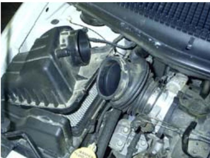
Next, disconnect the PCV tube and loosen the two hose clamps before removing the flexible coupling, air box lid and air filter. To remove the air box lid, simply release the two clips, one is at the side of the airbox and the other is at the back. At that point, you can tilt the lid of the airbox up (as pictured at left) and slide it to the side slightly to disengage the tabs from the base of the airbox to remove it. The air filter then just lifts right out of the base.
