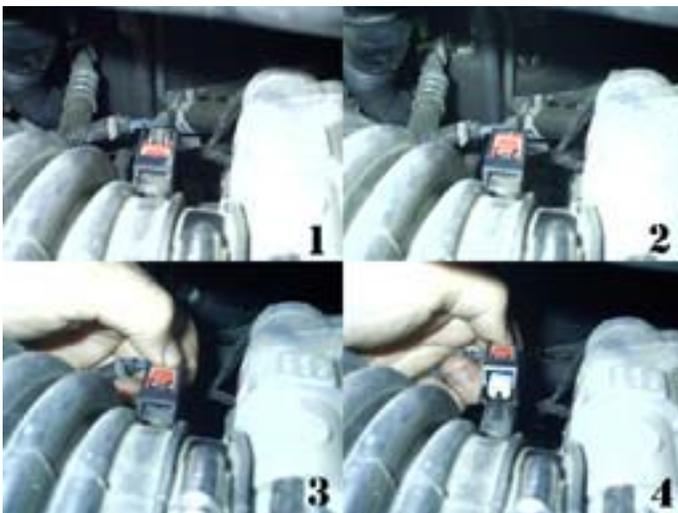
Disconnect the temperature sensor located at the back of the flexible coupling. To do this, you need to slide the red lock back, then you can squeeze the black lever at the back and unplug the connector.
