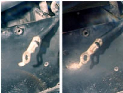
The stock battery cables have a tab at the end which is bent approximately 90 degrees. In order to attach the cable to the battery adapter brackets, it will be necessary to straighten out those tabs. A pair of pliers will do the trick.
