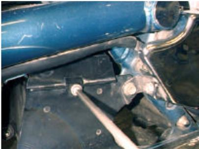
First, we must remove the old battery. To do so, use a Phillips head screwdriver to remove the screws holding the plastic battery box lid in place (there is one on each side), then slide the lid out of the bike from the right. There are slots in the front of the lid for the battery cables to pass through, so it will probably be necessary to work those out of the way prior to being able to slide the lid out.
