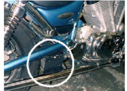
The Intruder's battery is located in a box just forward of the rear tire, as shown in the picture to the right.
