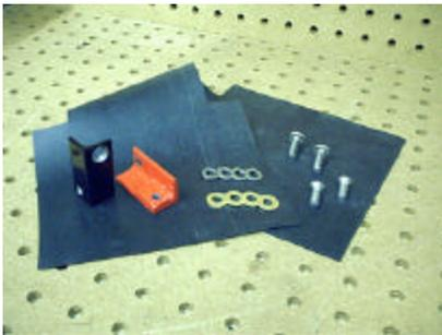
Pictured at left is the hardware included in the kit. The electrical contacts have been protected by a coating of dielectric grease. You can remove the excess prior to installing the adapters, but leaving some grease in place will help to ensure a good electrical connection.
