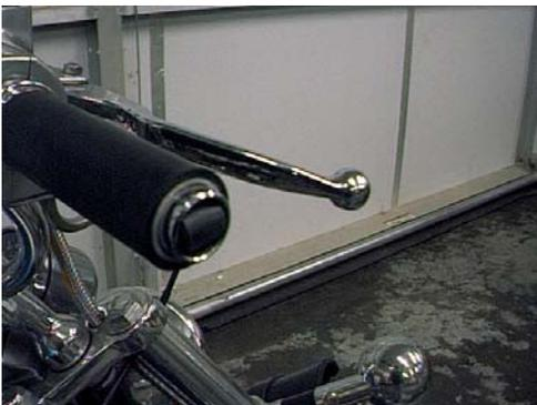
Next, either fold the remainder of the rubber strip up into the handlebar, or trim off the excess. **IMPORTANT: Be sure to leave enough rubber so that you can grab it, either with your fingers or a pair of pliers. If you don't have enough rubber to grab onto, removing the weight will be VERY difficult!**
