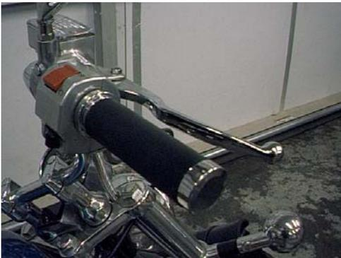
To the left is what we're starting with; a stock Suzuki Intruder handlebar. The first step is to remove the plastic "chrome" cap at the end of the grip. You should be able to simply pry it off with your fingers, though careful use of a screwdriver might be required if its stuck.
