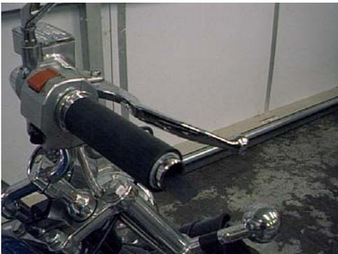
Once the cap has been removed, insert the strip of rubber so that approximately 1 to 1½ inches of the rubber is sticking out of the end. The rubber strips that are included have been purposely made "too wide". This is to allow for variations between handlebars. You will need to use a pair of scissors or a razor blade to make the strip thinner. (More on this later...)
