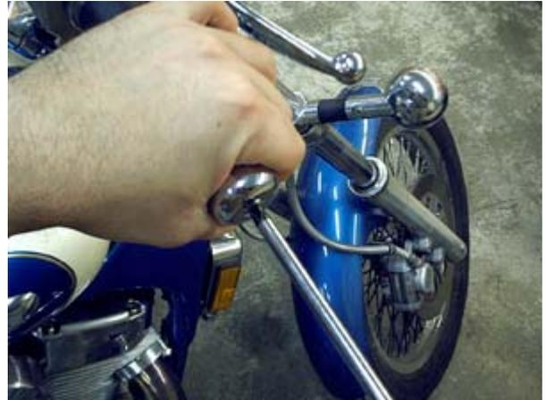
The above left photo shows our starting point; a stock Suzuki Intruder grip and bar end weight. The first step is to remove the stock vibration dampener assembly; you can do so by loosening the Phillips head screw at the end of the bar as shown in the upper right photo. Don't remove the screw completely (by doing so you run the risk of dropping parts of the stock assembly down into the handlebar); simply loosen it until you are able to slide the entire assembly out of the handlebar.
