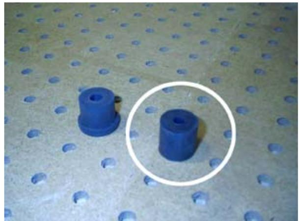
The stock vibration dampener assembly is shown in the above left photo. We need to re-use one of the rubber pieces from the stock assembly, so unscrew the nut at the end from the machine screw and remove the rubber piece. There are two pieces of rubber in the stock assembly; the piece we want is the one with the smaller diameter hole through its center and which does not have a ridge at one end; it is the same diameter throughout its length. It is circled in the photo at the above right.
