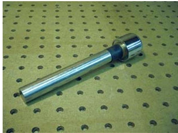
Attach the stock bar end weight to the Steiger Performance dampener as shown above. The supplied machine screw will go through the stock bar end, through the supplied shims, through the rubber piece from the stock assembly and finally will thread into the Steiger Performance vibration dampener. Don't tighten the screw with a screwdriver yet, just snug it up by hand and then slip this entire assembly into the handlebar.
