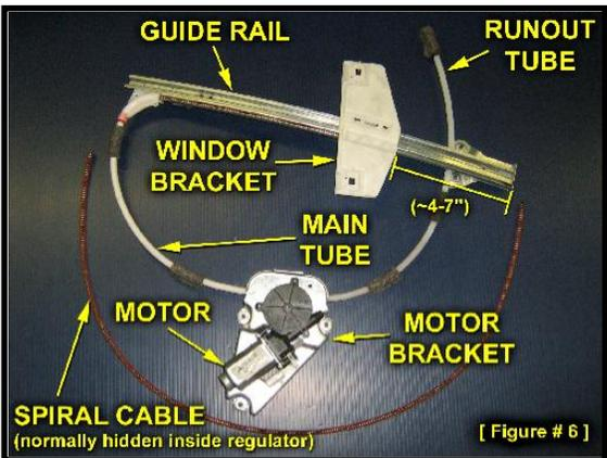
*Figure 6* shows what the window regulator assembly looks like when removed from the vehicle. Various parts of the regulator are labeled for your reference.
