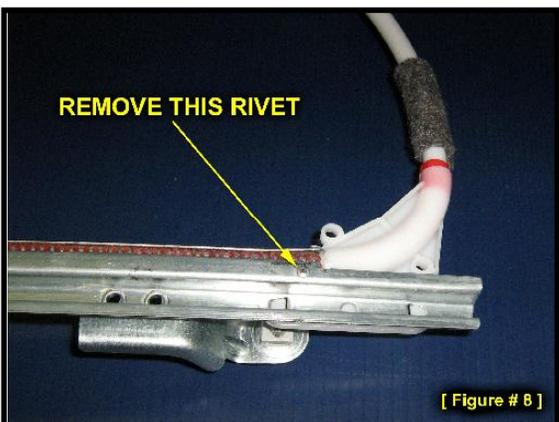
At the top of the guide rail (where the main tube attaches) you will find a small rivet. (*Figure 8*) Remove the head of this rivet. You can use a drill, grinder, cutoff wheel, Dremel® tool or even a hand file. A quick removal technique is to put the sharp edge of a chisel against the side of the head of the rivet and strike with a hammer. Whatever method you use, be careful to only remove the head of the rivet itself; do not damage the metal guide rail.
