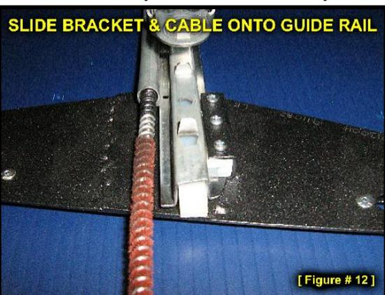
Slide the broken plastic bracket off the guide rail and install the replacement metal bracket as shown in *Figure 12*. The cable rides in the round channel, the nylon block in the middle of the bracket rides in the square channel and the nylon slot rides on the edge of the guide rail.
