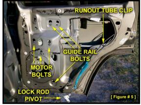
some additional space in the large opening to make it easier to remove the regulator from the door.
