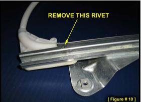
At the top of the guide rail (where the main tube attaches) you will find a small rivet. (*Figure 10*) Remove the head of this rivet. You can use a drill, grinder, cutoff wheel, Dremel® tool or even a hand file if you have the elbow grease to spare, but whatever method you use, be careful to only remove the head of the rivet itself; do not damage the underlying metal guide rail.
