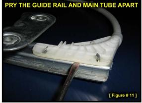
the main tube that is facing up in Figure 11 should be facing down while you press the rivet through.)
