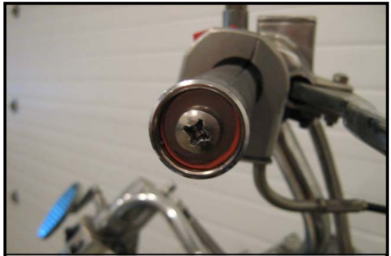
Step 3: Insert into bar and tighten screw
