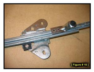
into the guide rail to verify that the repair bracket didn't move while you were tightening it. Next, you need to thread the spiral cable into the repair bracket. Before doing so, you must remove approximately one inch of the "fuzz" from the end of the cable. (A wire wheel mounted on a bench grinder works great for this, or you can use a wire bristle brush, or if all else fails, just pick it out with a pair of tweezers or needle nose pliers.)
