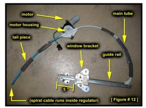
(usually silver) and the third is different (usually gold). The same/silver bolts go in the outside holes, and the different/gold one through the middle hole. Thread the regulator back into the door, reversing the method you used to remove it. Slide the motor and guide rail into their respective slots and tighten the nuts. (The tail piece should run underneath the lower guide rail bracket, not above it.) Plug the motor back into the wiring harness
