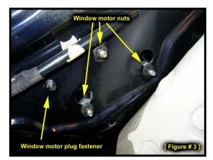
nuts as well as the bolt at the top of the guide rail and the two bolts at the bottom of the guide rail. You do not need to completely remove the nuts on the motor or the bolts on the guide rail, just back them out 1/4" or so. Slide the motor up enough for the nuts to pass through the holes at the top of the slots they are resting in, then rest the motor on the bottom of the door and let it sit there for now.
